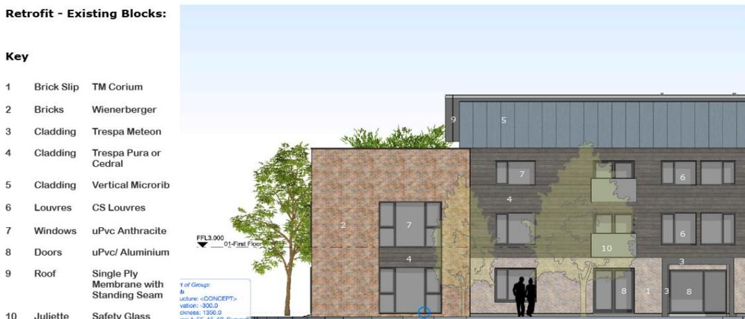
Figure 7 materials to Existing and New build blocks
