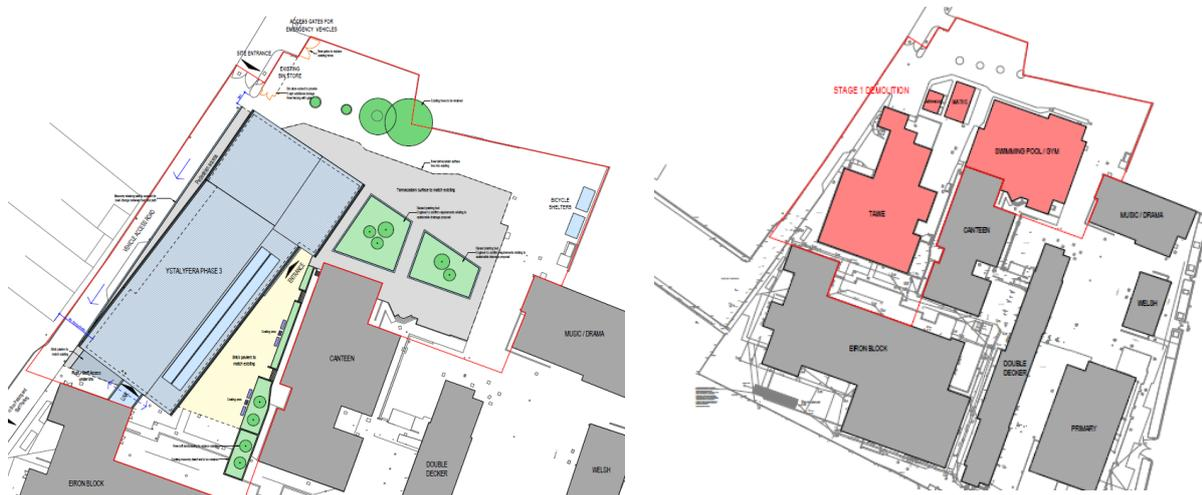
The footprint of the building shown on the plan on the left, with the existing buildings to be demolished on the right, highlights how the reduction on floor space, accommodates additional areas of open space and play area.
