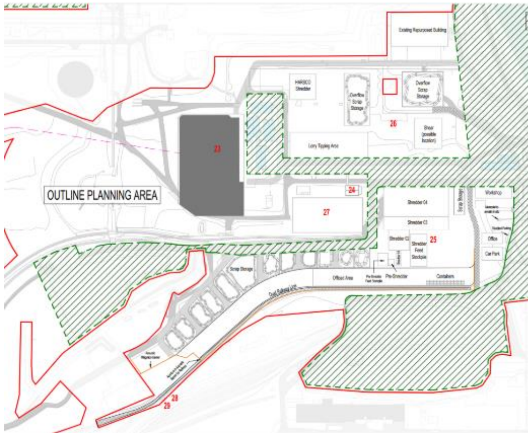
Figure 11: Extract of ES Figure 2.1c showing the illustrative scrap handling facilities within the outline planning application area for phase 2.
